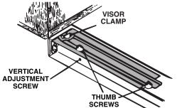
The visor slides each have a screw for adjusting the height of the visor trim, if necessary. The vertical adjustment screw allows the top and bottom edges of the visor trim to be matched with the control trim.
