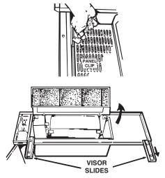
Pull the visor slides out. Rotate the panel clips and swing the panel open.
