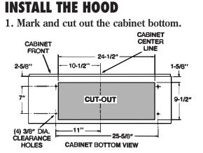
Prepare the cabinet bottom as shown above. Be sure to locate the cut-out and four holes from the front of the cabinet to ensure a flush mount.
