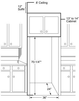
\*The rough-in dimension of 70-1/4" is minimum and is measured from the finished floor to top of opening (or the underside of the overhead cabinets). For Models with Trim Kit: If trameless style cabinets are planned for above the refrigerator, you may need to consider adding a maximum of 1/4" (70-1/2") to height of opening to allow additional clearance between cabinet doors and top of refrigerator trim when cabinet doors are in open position.
