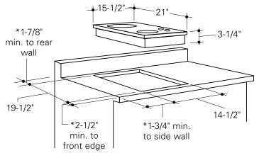
\* When installed, the following minimum clearances must be maintained: 2" from front of cooktop to front edge of countertop. 1" from back of cooktop to rear wall. 1" from side of cooktop to side wall.
