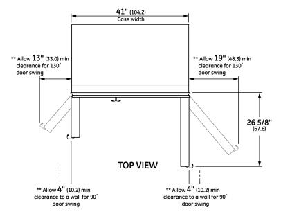
\*\* These refrigerators are equipped with a 2-position door stop. The factory-set 130° door swing can be adjusted to 90° if clearances to adjacent cabinets or walls is restricted. Allow full 130° door swings for pan removal. If the 90° door stop position is used, pan access is maintained, but pan removal is restricted.
