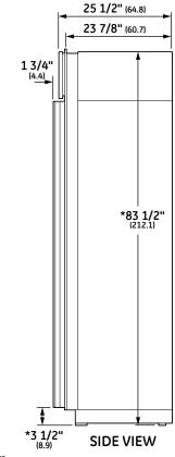
\* Shipping height. Use leveling legs and wheels for maximum 1" height adjustment from shipping height.
