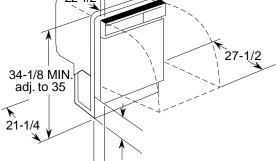
Installation Information (in inches) Countertop This wall area must be free of . 90° 90 pipes or wires 24" 2 MIN. Electrical wiring is 3" from cabine Hot water Electrical 34-1/2±1/4" Underside line on wiring on left right of countertor to floor Plumbing and electrica service must enter inside shaded area 24" MIN.
