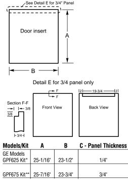
\*GPF800 Heavy Spring Kit required for custom door panel weighing more than 4 lbs.
