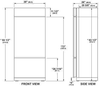
\* Shipping height. Use leveling legs and wheels for maximum 1" height adjustment from shipping height. Nominal installation height is 84"
