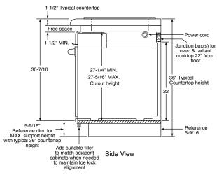
This installation is to achieve minimum gap between bottom of countertop and control panel.
