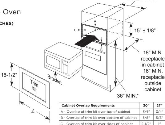
\*For ADA compliance, the microwave must be installed no higher than 37-7/8".
