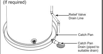
**NOTE:** Auxiliary catch pan MUST conform to local codes. Catch Pan Kits are available from the store where the water heater was purchased, a builder store or any water heater distributor. The catch pan should be 2" (5.1 cm) minimum larger than the Water Heater base diameter. To prevent corrosion and improve Drain Valve access it is recommended that the water heater be placed on spacers inside the catch pan.
