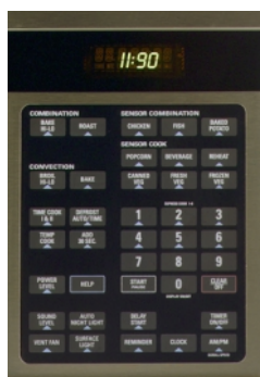
Combination Bake/Hi uses 30% microwave power, combined with convection cooking for faster cooking results.
