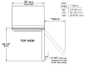
\*\* These refrigerators are equipped with a 3 position door stop. The factory set 115° door swing can be adjusted to 90° if clearances to adjacent cabinets or walls is restricted. Allow full 130° door swings for pan removal. If the 90° door stop position is used, pan access is maintained, but pan removal is restricted.
