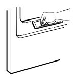
**The Exhaust Duct:** Inspect and clean the exhaust ducting at least once a year to prevent clogging. A partially clogged exhaust can lengthen the drying time.
