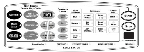
NOTE: Any time you make a selection that is incompatible with the chosen dry cycle, the dryer will beep twice.
