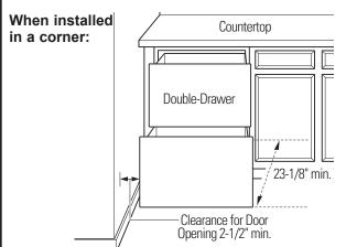
Allow 2-1/2" min. clearance between Double-Drawer and adjacent cabinet, wall or other appliances. Allow 23-1/8" min. clearance from the front for drawer opening.
