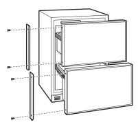
Custom handles of your choice, supplied by your cabinet maker, must be installed onto the overlay panels before they are slid into the trims. Countersink all screws into the backer panels. Screws cannot protrude from the backer panels.
