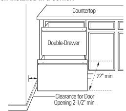
Allow 2-1/2" min. clearance between Double-Drawer and adjacent cabinet, wall or other appliances. Allow 22" min. clearance from the front for drawer opening.
