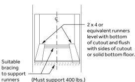
**JKD5000** Cabinet 27" A - Overlap of oven at top of cutout 1" B - Overlap of oven other side of edge of cutout 1" C - Overlap of oven at bottom of cutout 1" Oven D - Install depth 23 1/2" E - Overall height with trim 49 11/16" to 50 1/8" F - Overall width 25 1/4"
