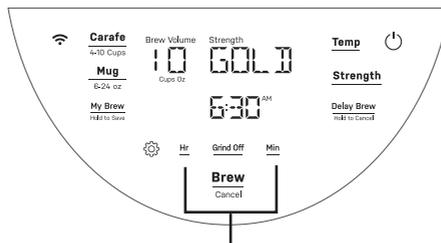
Press and Hold the Hour and Minute buttons to turn on/off WiFi.
