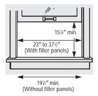
Window opening dimensions are for a standard double-hung window.
