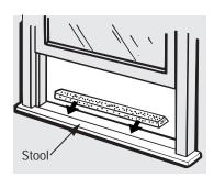
5 Using the level, adjust the leveling bolt so the curved top of the support bracket is 1/4" below the top of the window stool.
