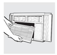
The air filter is behind the front grille insert and should be checked and cleaned at least every 30 days or more often if necessary.
