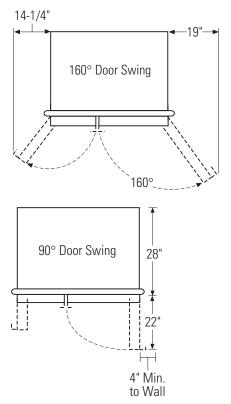
Allow 19" minimum clearance on the fresh food side for a full 160° door swing and pan removal. Allow 14-1/4" clearance on the freezer side for removal of ice bin.
