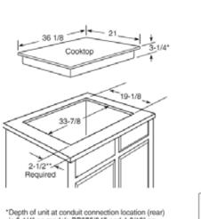
Depth of unit at conduit connection location (rear) is 6-11/4" on models PP975/945 and 4-3/16" on models CP350/650, PP944/962/932/912, and JP656/356/336. Depth of unit at baffle (front) is 4-5/8" on models PHP960/900.
