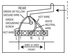
POWER SUPPLY CORD 4 #10 AWG MINIMUM COPPER CONDUCTORS, 30 AMP, 240V, WITH CLOSED-LOOP TERMINALS TYPE UL RECOGNIZED MINIMUM RATED 90°C.
