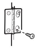
Remove the remaining screws from the side of the opening from which the door was removed. With these screws, secure each hinge at the bottom. Tighten the two top screws of each hinge. Reinsert the plastic plugs on the side from which the door was removed.
