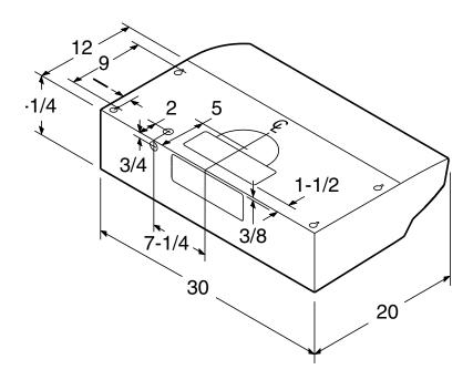
Exhaust outlet connects to 3/1/4" x 10" duct (vertically or horizontally) and 7" round (vertically). Includes rectangular damper and 7" round damper adapter.
