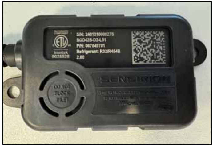
FIGURE 10. Example of Clear, Unobstructed Sensor Inlet
