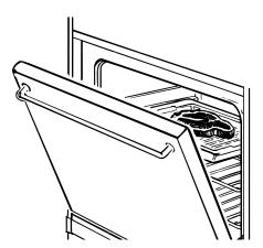
Leave the door open to the broil stop position. The door stays open by itself, yet the proper temperature is maintained in the oven. **NOTE:** Food can be broiled with the door closed, but it may not brown as well because the oven heating element will cycle on and off.
