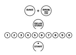
When the display shows  $\supset$  the oven is set in Sabbath. When the display shows  $\supset \subset$  the oven is baking/roasting.
