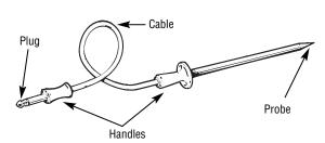
The temperature probe has a skewer-like probe at one end and a plug at the other end that goes into the outlet in the oven.
