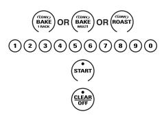
When the oven starts to heat, the changing temperature, starting at 100°F, will be displayed. When the oven reaches the temperature you set, 3 beeps will sound.
