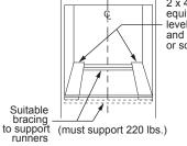
2 x 4 or equivalent runners level with bottom of cutout and flush with sides of cutout or solid bottom floor.
