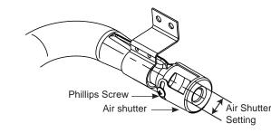
With a Phillips head screwdriver, loosen the screws securing the air shutters on the burners and adjust the air shutters according to chart.
