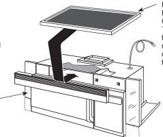
Filter Kit JX81L— Recirculating Charcoal Filter Kit To be used when the Spacemaker microwave oven cannot be vented to the outside.
