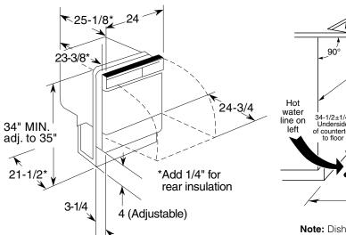
Countertop This wall area must be free of 90° pipes or wires 24" MIN. Electrical wiring is 3" from cabinet Electrical 34-1/2±1/4" Underside of countertop to floor wiring on right Plumbing and electrical service must enter inside shaded area 24" From 9" MIN, from wal White (neutral) Ground Black (line) 24" MIN.
