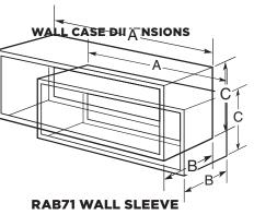
Heavy-gauge galvanized steel, with insulation. A  $\,$  – 42", B – 13-3/4", C – 16"
