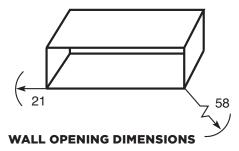
Add 1/4" to A and C dimensions for all cut-out size. RAB71 16-1/4" Min. H x 42-1/4" Min. W RAB71 available in 16", 24", 28" and 31" depths RAB77 16-1/2" Min. H x 42-3/8" Min. W
