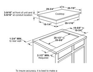
template when cutting the opening in the counter
