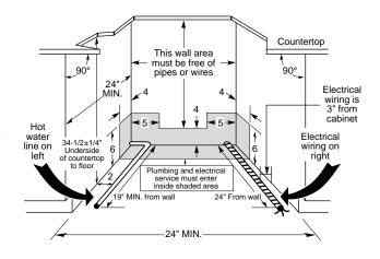
**Note:** Dishwasher must not be installed more than 10' from sink for proper drainage. All plumbing and electrical work must be in accordance with local codes. Dishwasher includes drain hose and leveling legs.
