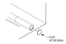
Connect standard metal elbows and ducts to complete the exhaust system. Cover back opening with a plate (Kit WE1M454) available from your local service provider. Place dryer in final location.
