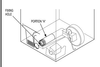
Reconnect the cut portion (A) of the duct to the blower housing. Make sure that the shortened duct is aligned with the tab in the base. Use the screw saved previously to secure the duct in place through the tab on the appliance base.
