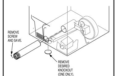
Detach and remove the bottom, right or left side knockout as desired. Remove the screw inside the dryer exhaust duct and save. Pull the duct out of the dryer.
