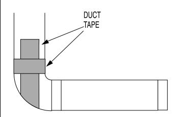
CAUTION: Internal duct joints must be secured with tape, otherwise they may separate and cause a safety hazard.
