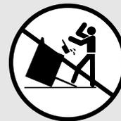
To check if the device is installed and engaged properly, carefully tip the range forward. The Anti-Tip device should engage and prevent the range from tipping over.
