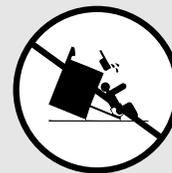
If you pull the range out from the wall for any reason, make sure the device is properly engaged when you push the range back against the wall. If it is not, there is a possible risk of the range tipping over and causing injury if you or a child stand, sit or lean on an open door.
