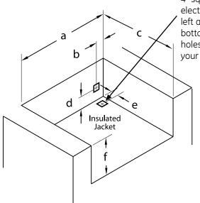
4" square holes for gas and electrical connections both left and right sides (rear or bottom access). Make these holes in the frame based on your requirements.
