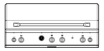
Monogram grills are factory-set for Natural or LP gas operation. Be sure to order the correct model for the installation situation.
