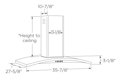
\*The supplied duct cover fits 7'11" to 10'4" ceiling heights (10'9" in recirculation mode).
