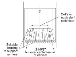
(Platform must be able to support cabinet load, weight of oven, and additional oven loads)
