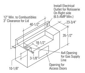
36" wide models: Installation in a non-combustible enclosure.
