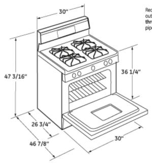
Recommended area for 120V autiet on rear wall and area for through-the-wall connection of pipe stub and shut-off valve.
