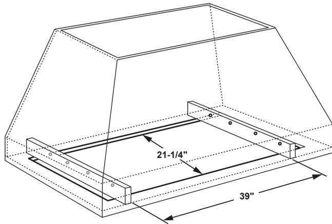
These hoods are secured to the custom cabinet from both sides through 8 screws. Two 2x4 studs separated by 39" need to be provided on the custom cabinets for installation.
