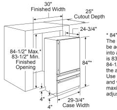
\* 84" High installation. The refrigerator can be adjusted to fit into a cutout that is 83-1/2" min. to 84-1/2" max with the appropriate door kit. Use leveling legs and wheels for a maximum 1" height adjustment.
