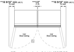
\*\* Dimensions based on handle height of 2 9/16" (6.5) \*\*\* Included in the 59 1/2" or 71 1/2 cut out requirements
