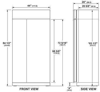
\* Shipping height. Use leveling legs and wheels for maximum 1" height adjustment from shipping height. Nominal installation height is 84".
