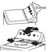
**3.** Remove the five screws from the control panel back cover. The conversion kit is now accessible.
