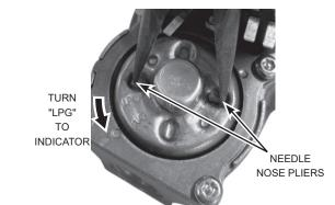
Rotate the dial counterclockwise, lining up "LPG" marking with the indicator on the gas valve.
