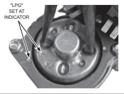
**8.** Using a 3/8" wrench, remove the NG burner orifice from the gas valve assembly turning it counterclockwise. Install the LP orifice from this kit.
