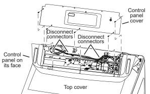
Disconnect the connectors from the control board and set the control panel aside.
