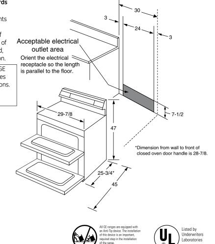
\*Note: Check local codes for required breaker size.
