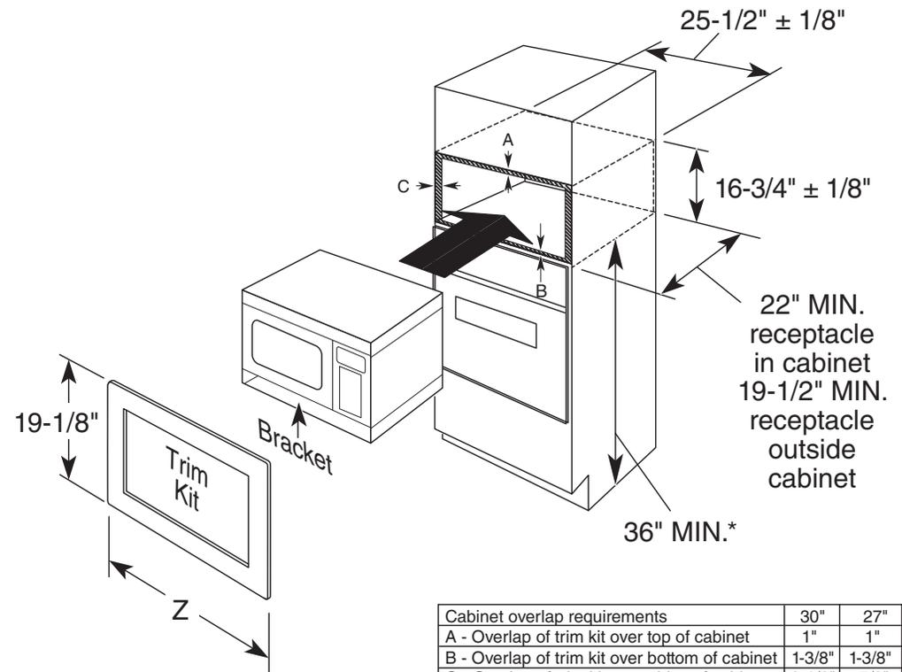
\*For ADA compliance, the microwave must be installed no higher than 36-1/4".
