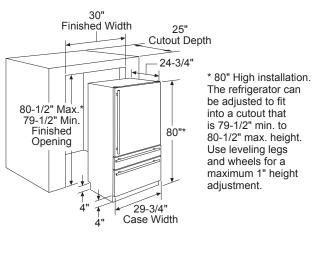
The refrigerator can be adjusted to fit into a cutout that is 79-1/2" min. to 80-1/2" max. height. Use leveling legs and wheels for a maximum 1" height
