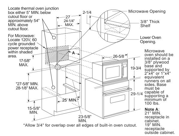
**Note:** Recommend approximately 1/4" gap between microwave trim and wall oven trim. (The 2-1/4" dimension should create a 1/4" gap.) Allow 1-1/2" for overlap of the Microwave Oven Kit Trim over all edges of the trim kit cutout.
