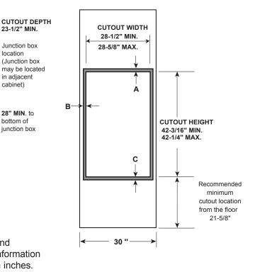
ATTENTION INSTALLER: All electric wall ovens must be hard-wired (direct-wired)
