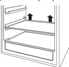
To remove, lift up on the back of the shelf
