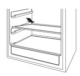
Place in slots when replacing the shelf
