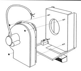
Step T Finalize Installation  Place the cover over the the assembled kit and secure with 16 screws.
