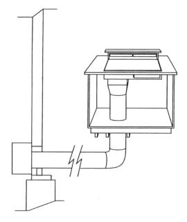
The blower and motor assembly can be mounted on an outside wall. This kit provides a means to mount the blower outside with a protective cover.
