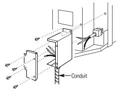
2 If a fuse and fuseholder are to be used, the knockout at the top of the box is for mounting a Buss Fuseholder. Be sure the fuse and fuseholder are of the same rating as the branch circuit.
