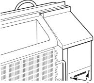
Remove screws and panel to access terminal connections
