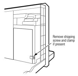
**3** Remove the room cabinet by pulling it out at the bottom to release it (1), then lift it up to clear the rail along the unit top (2).
