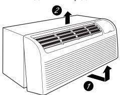
**To replace:** Place the tabs over the top rail (1). Push inward at the bottom until it snaps into place (2).
