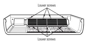
Remove the room cabinet and flip the louver insert to change the air direction.
